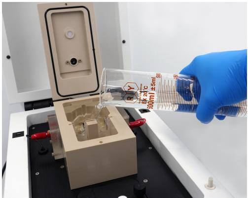
8. Ensure that there is water in the device and do not run the pump dry. Press "Auxiliary Power" on the touchscreen. This will turn on the liquid pump, sample cup mixing, and sample cup rotation. Upon startup the Chamber Hex Piece will rotate faster than normal for 5 seconds to allow you to visually verify that the Hex Piece is indeed rotating. The software will also deactivate so that power cannot be cycled too quickly for some components.
