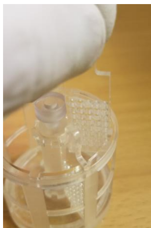
Insert sample holder spacers in sample holder.
