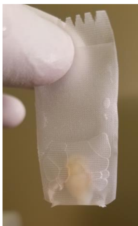
Insert sample in mesh bag with long axis vertical.
