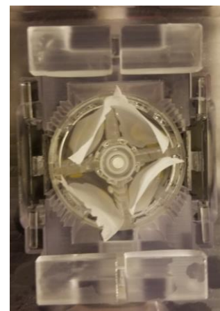
Insert sample holder into the clearing chamber
