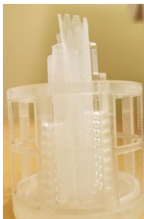
Insert mesh bags into sample holder.
