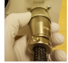
SCREW BEARING LOCK NUT CLOCKWISE COMPLETELY.
