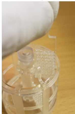
Insert sample holder spacers in sample holder.
