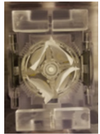
Insert sample holder into the clearing chamber.
