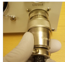
ALIGN TABS AND PLUG IN CABLE
