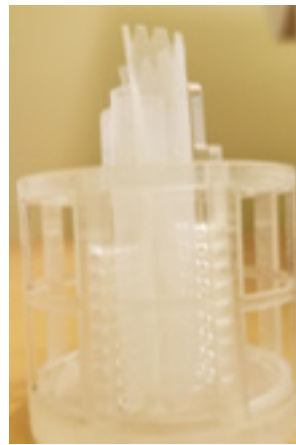
Insert mesh bags into sample holder.
