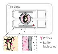
Nanoporous membrane retains antibodies inside sample chamber and protects against contamination (Kim, PNAS, 2015).
